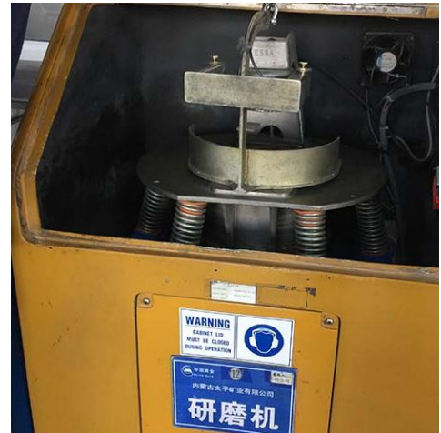
Onsite pulverization machine
